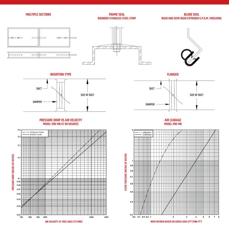
NOTE: Pressure drop and infiltration tests performed by Air-Ins Laboratories on a 48" x 48" damper section, in accordance with the AMCA 500 standard.
