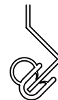
Weather strips -BLADE TIGHT DAMPER (212 °F / 100 °C) EXTRUDED E.P.D.M RIGID AND SEMI RIGID MOULDING
